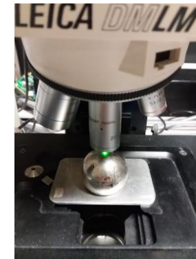
Raman Spectroscopic measurements for CoCrMo implant surfaces with SF Lubricant
