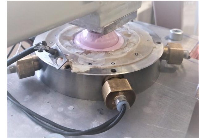
Ball-on-cup Configuration within hip joint simulator
